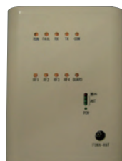
Network coupler RS-1200CPF RS-1200CPA It is connected LAN cable.
